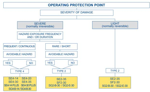
Note: The given information is indicative and synthetic; it is compulsory to refer to the complete EN 954 standard for a correct risk and safety type evaluation.
